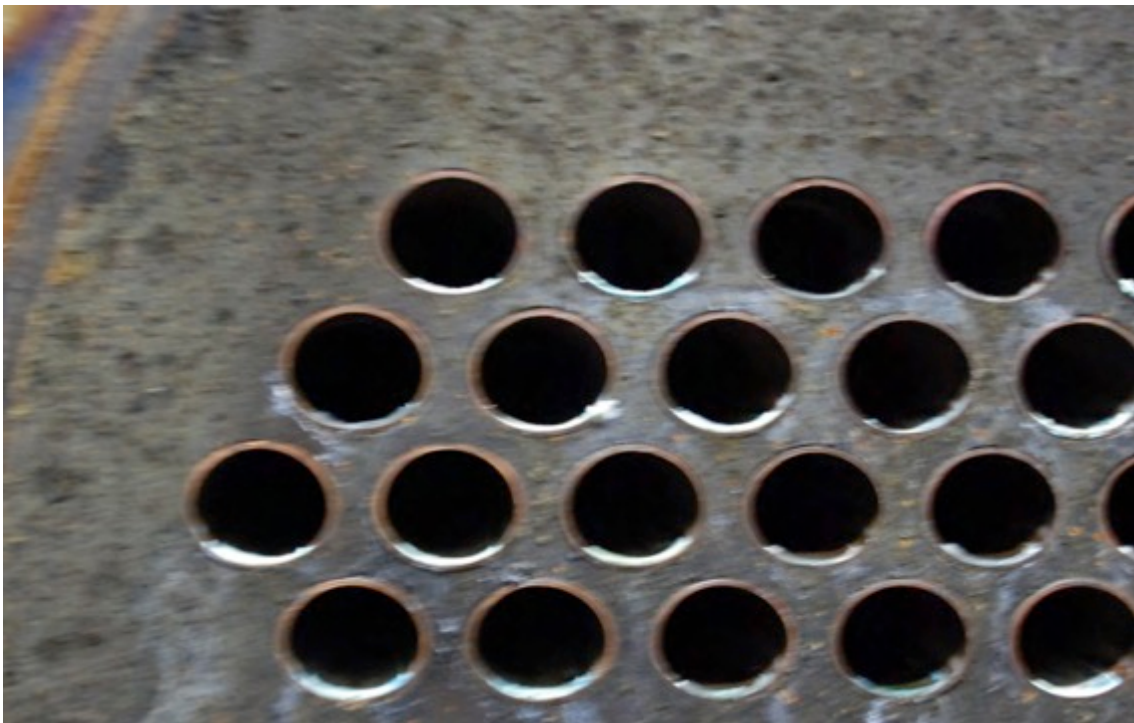
Chiller tubes from phase one test facility after two cooling seasons on ProMoss™
