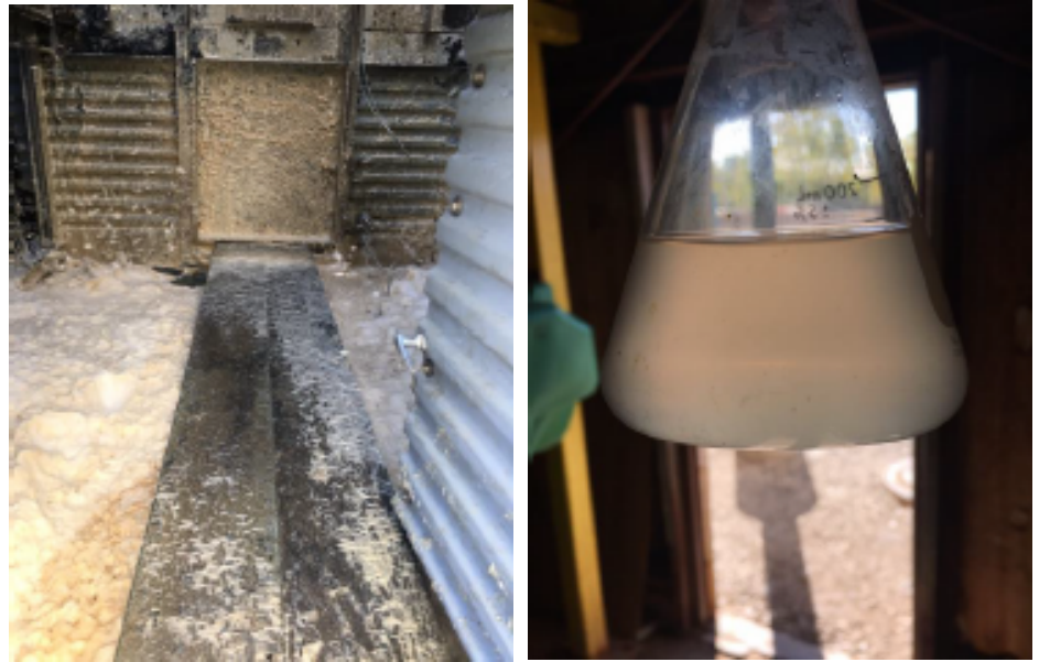
Fig. 1 Before ProMoss™: Water heavily contaminated with product from process systems and microbial growth. Thick organic contamination build up. High turbidity and heavy foaming.
