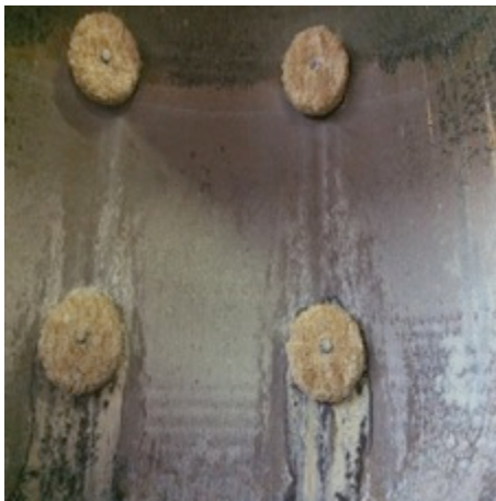
Figure 5. The only visible scale formation was on the zinc anodes. Scoping the tubes showed no scale or corrosion. The scale was analyzed and was zinc oxide.
