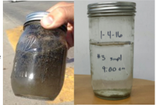
Oil contaminated cooling water
