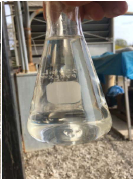
Fig. 2 After 1 month of ProMoss™ being added to treatment: Water clarity improved dramatically. Foaming minimal. No new organic contamination formation.
