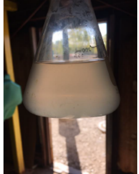
Fig. 1 Before ProMoss™: Water heavily contaminated with product from process systems and microbial growth. Thick organic contamination build up. High turbidity and heavy foaming.
